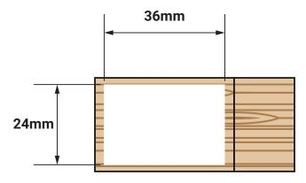
PRINTABLE AREAUSB DIMENSIONS36mm x 24mmL: 59.5mm x W: 9.5mm x H: 28mm
